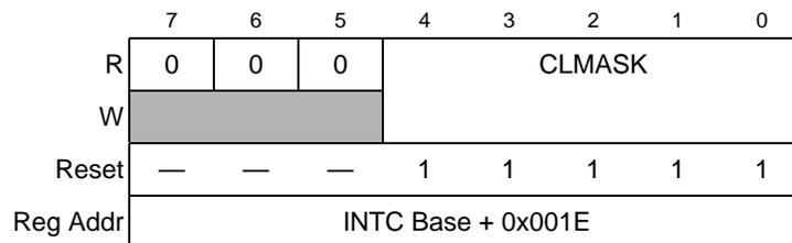
Figure 10. INTC Current Level Mask Register (CLMASK)
