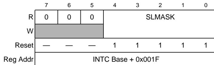
Figure 11. INTC Saved Level Mask Register (SLMASK)
